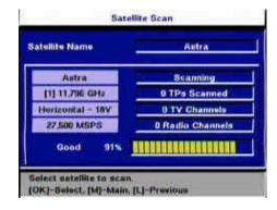
The signal quality and the scan progress are indicated during the scan.
